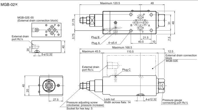
For products with option code G, the pressure adjusting screw is located at the port A side.
